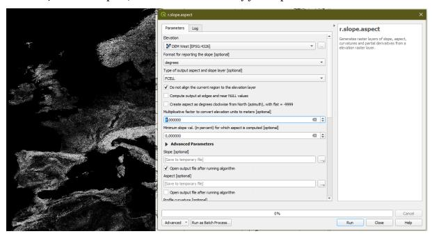
This results in a map no longer showing how high the terrain is, but how steeply rugged it is. Note the high plains of Spain and Morocco, for example: they are no longer grey (for being high), but black (for being plain).
